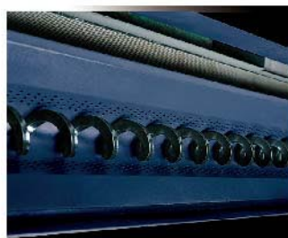
Automatic chip removal (Screw type chip conveyor)
