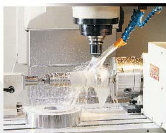
High pressure coolant (P:3.5 kg/cm 2 , Q:100 l/min)
