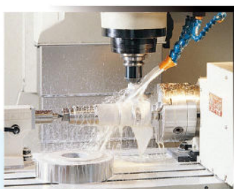
High pressure coolant (P:3.5 kg/cm 2 , Q:100 l/min)
