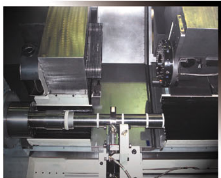
Option Application- LH: Grinding Head RH: Y Axis+Power Turret Steady Rest (Auto Self-centering)
