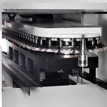
Magazzino a catena mobile Movable chain magazine
