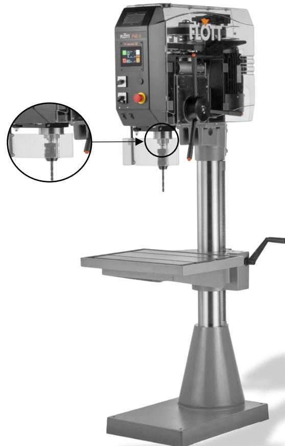
Universal drill with infinitely variable speed drive,
